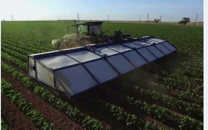
Figure 28. Blue River Technology's AI powered 'See & Spray' system
