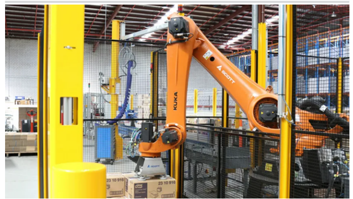
Figure 12. SCT—Robotic palletising cell stacks cases onto pallets
