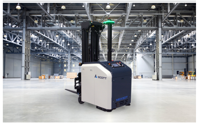
Figure 14. SCT—NexBot AGV transports finished pallets
