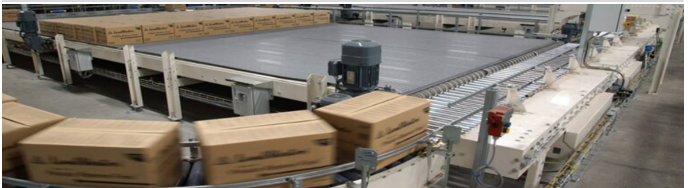
Figure 3. SCT—AccuTable buffers products ahead of palletisation
