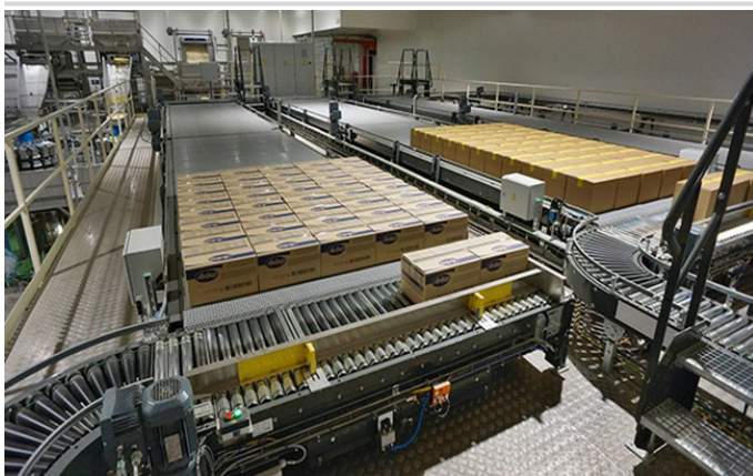
Figure 13. SCT—AccuTable buffering within a multiline palletising system
